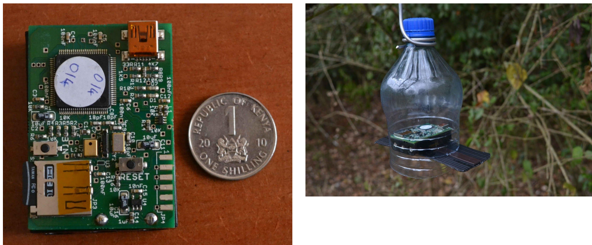
Figure 3: The acoustic recorder in the lab (left) and installed in the field (right)
